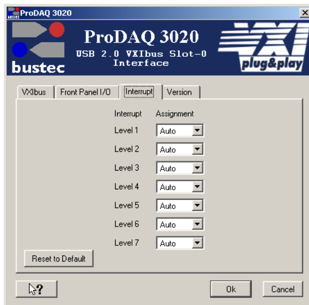
Figure 15 - Configuring the Interrupt Lines
